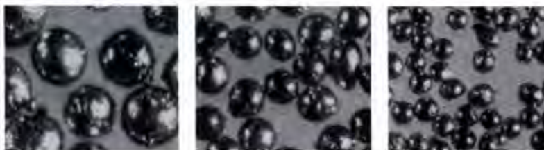
Shown above are photographs of Handy & Harman's Sil-Fos 5 powder, in three standard mesh sizes. Photographs are all enlarged 100 times. Note consistency of particle size and shape in all three sizes.
