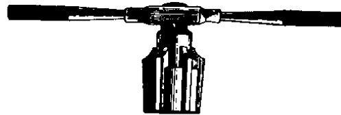
(B) Adjustable tap wrench used for any size taps. Shown with tapered reamer that is sometimes used before tapping.
